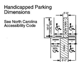
in width in addition to an 8 foot access aisle); or 24 feet by 18 feet for a double van space, or a non-van and van double space (8 feet in width for each space with an 8 foot access aisle between spaces).
